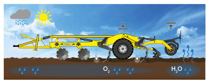
Loosening with raised packers = faster drying (driving on the axle on waterlogged ground)
