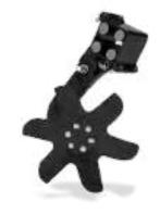
ACTROS can be equipped with levelling disc section with a diameter of 460 mm. The discs level soil after the working shares and before the rear packers. The field is perfectly levelled. Suitable mainly for heavier soils.
