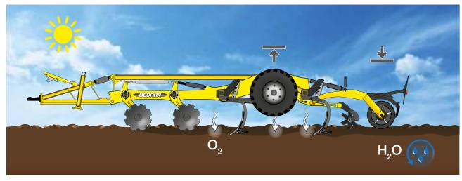
Loosening with compaction (driving on rollers)
