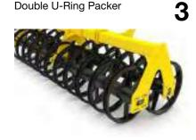
A double-row steel packer with a self-cleaning effect, excellent crumbling and low stickiness thanks to the U-shaped ring.
