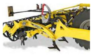
The share working depth is set hydraulically using hydraulic clips on the rear rollers.
