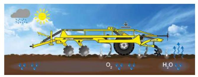
Loosening without rollers = faster drying (driving on the axle in waterlogged soil)
