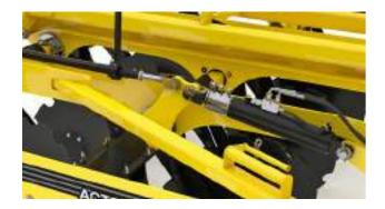
The disc working depth is set hydraulically using hydraulic clips.
