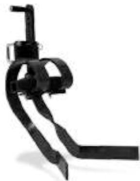
The basic ACTROS equipment includes spring levelling section that level the soil after shares. Suitable mainly for lighter soils.
