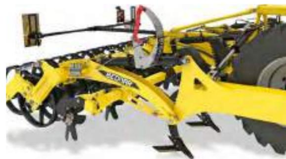
The share working depth is set hydraulically using hydraulic clips on the rear rollers.
