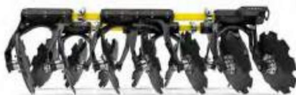
The discs are 42 cm apart and they work at an angle of 11° (front) and 9° (rear).
