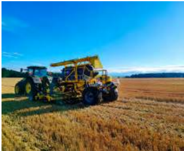
DIRECT SEEDING OF CATCH CROPS INTO STUBBLE AFTER WINTER WHEAT HARVEST
