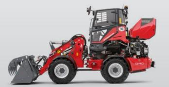
overhead guard eps and a cabin are available. The selection of the right driver's cab allows maximum flexibility for different applications and boundary conditions.
